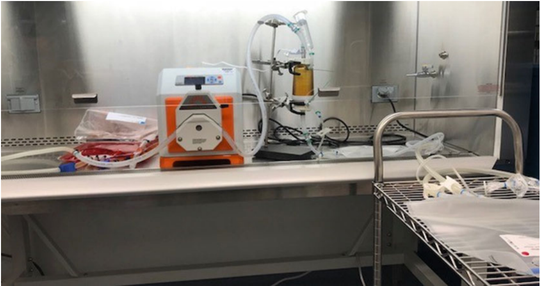
Fig. 2 Photo of the completely assembled Mustang Q capsule with pump and bioprocessing bag attachments
