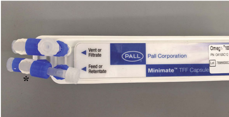
Fig. 2 TFF using the Minimate™ capsule equipment setup. (a) One piece of tubing connects the sample reservoir to the feed port of the Minimate™ capsule passing through the pump. The product flows parallel (tangential to) the membrane. The pressure generated by the flow stream causes liquid flow through the membrane (permeate). Another piece of tubing circulates the retentate back to the sample reservoir. The filtrate (permeate) is discarded. Flow direction of the sample is indicated by yellow arrows. Top (b) and side (c) view of the capsule showing feed port (marked with an asterisk) and exit port for permeate (red arrow)
